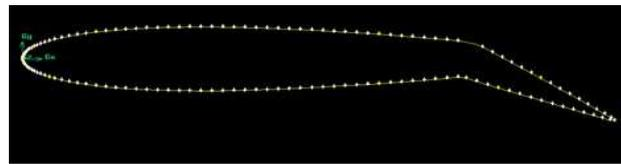
Figure 5: Morphed Aileron Deflected 25 Degree Down
