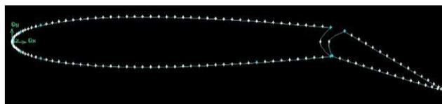
Figure 6: Un-morphed Aileron Deflected 25 Degree Down
