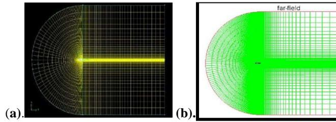
Figure 4: Meshed Airfoil Window in GAMBIT (a) and Fluent (b)
